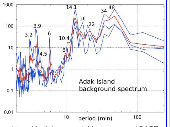
TEDA has been applied to data provided by NOAA/PMEL (USA) registered both by coastal tide-gauges and DART buoys. Here we present the results of the application of TEDA to data registered by the coastal tide-gauge installed at Adak Island, Alaska, USA, which is a station that keeps track of several historical tsunamis.
